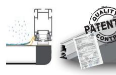
• The PVC offers stiffness on the guide hook to seal onto to the guiderail. • The plasticized polyethylene gives elasticity to the parts that are in contact with the fabric to avoid PVC memory effect from temperature variation. The patented double fin structure assures that rainwater is routed into the unit's integrated gutter and does not sill over the sides even in windy
